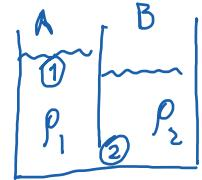
$$P_{atm} + \frac{1}{2} \rho_1 v_1^2 + \rho_1 g h_1 = p_2 + \frac{1}{2} \rho_1 v_2^2$$
